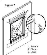
Note: Unit must be installed square, plumb and level or warranty may be void.
